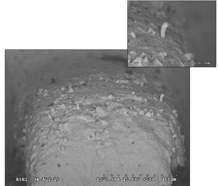
Whisker on termination finish (LF card)
